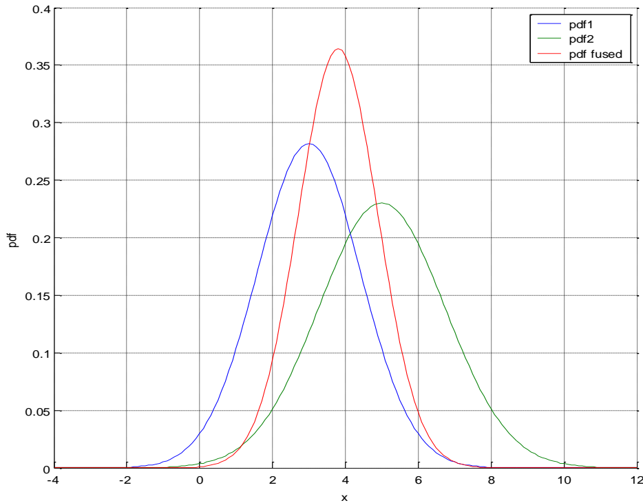
Picture 2-4: graphic example of what can be, in the scalar case, the previous distribution, the likelihood function and the posterior distribution. The posterior distribution has as average the average weighted among the original averages and has a lower variance than both the original ones, in fact, it has more information than the individual contributions.
