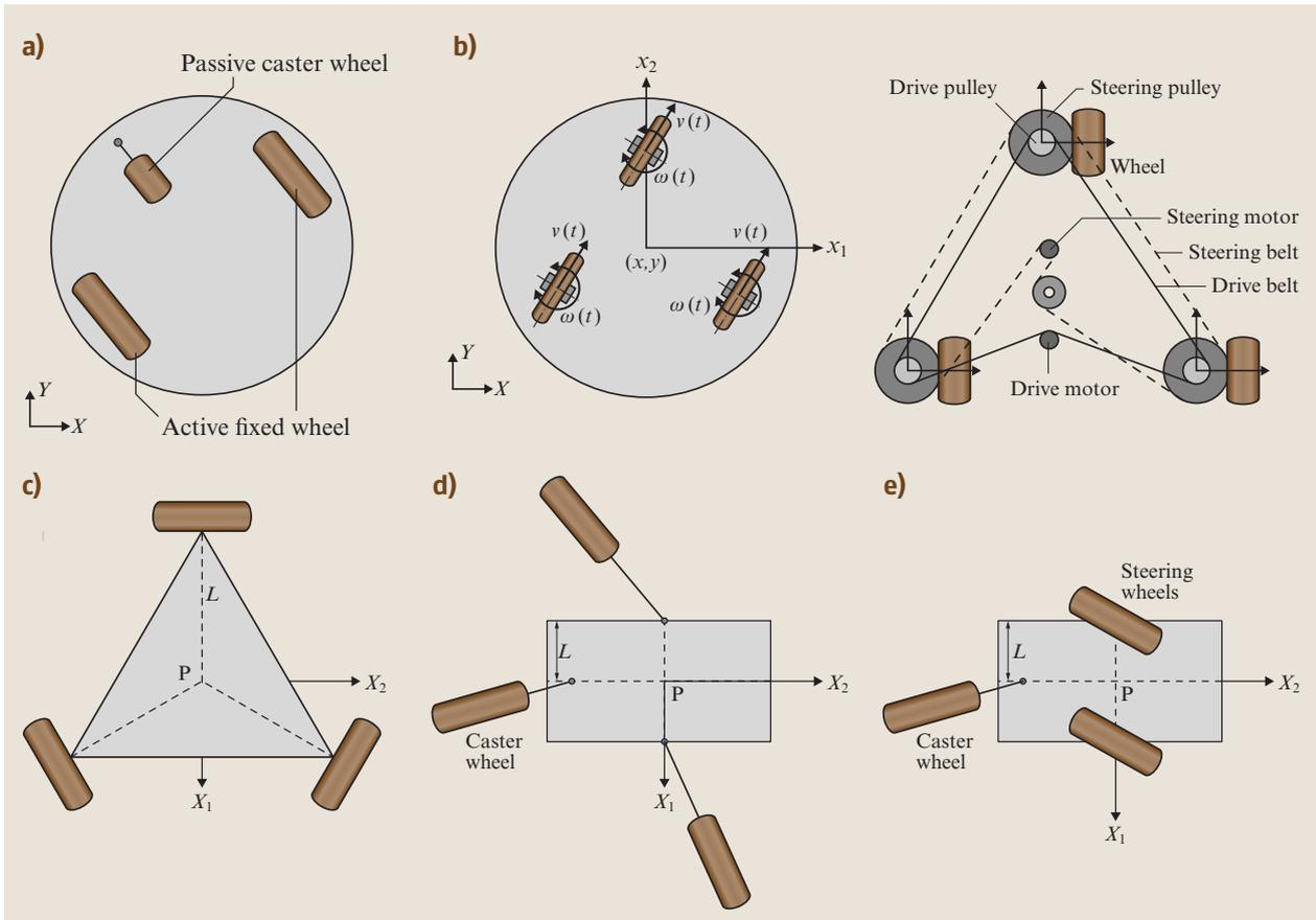
**Fig. 17.7** (a) Two-wheel differential drive, (b) synchronous drive, (c) omnimobile robot with Swedish wheels, (d) omnimobile robot with active caster wheels, (e) omnidirectional robot with active steerable wheels
