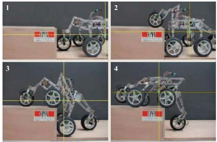
Fig. 17.9 A mobile robot for rough terrain [17.18]
