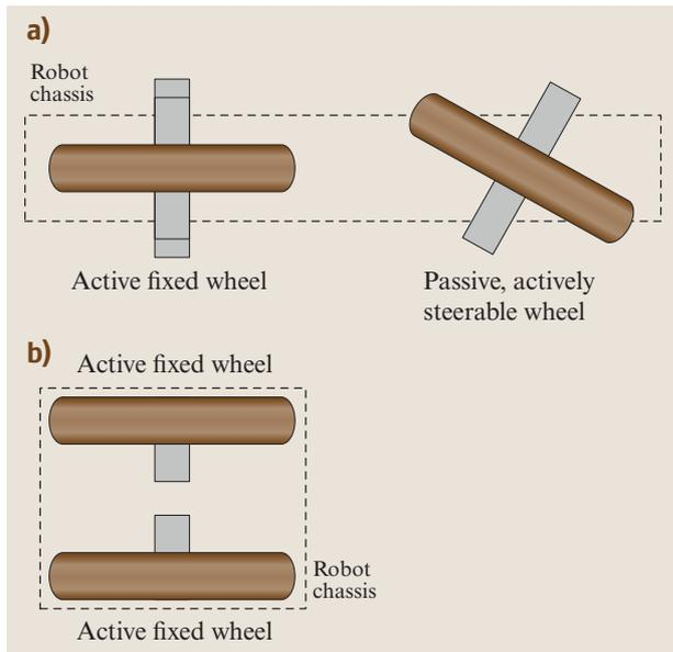
**Fig. 17.6** (a) Bicycle-type robot, (b) inverted-pendulum-type robot
